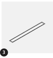
Cut floor covering and/or use flexible sealants to make good floor surface for a flush finish.
